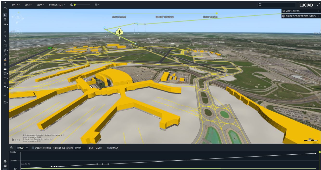
Figure 11 - AIXM 5 data and flight plan preview in 3D with vertical view.
