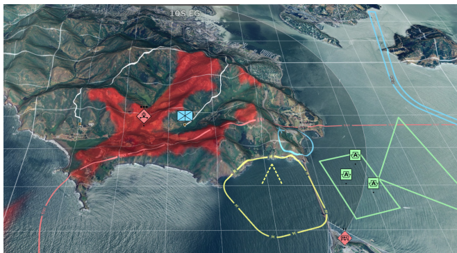
Figure 5 - Line-Of-Sight (LOS) analysis and LOS routing on 3-D terrain
